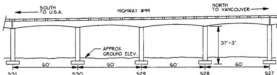
Figure 1. Typical Four Span Segment of Oak Street Bridge.
