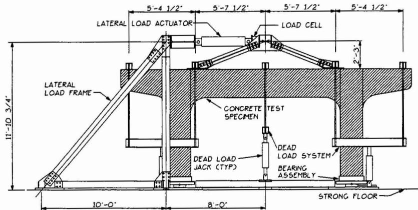
Figure 2. Typical Test Arrangement.
